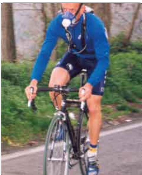
For comfortable biking K4 b 2 can be placed on the back of the subject by adjusting harness
